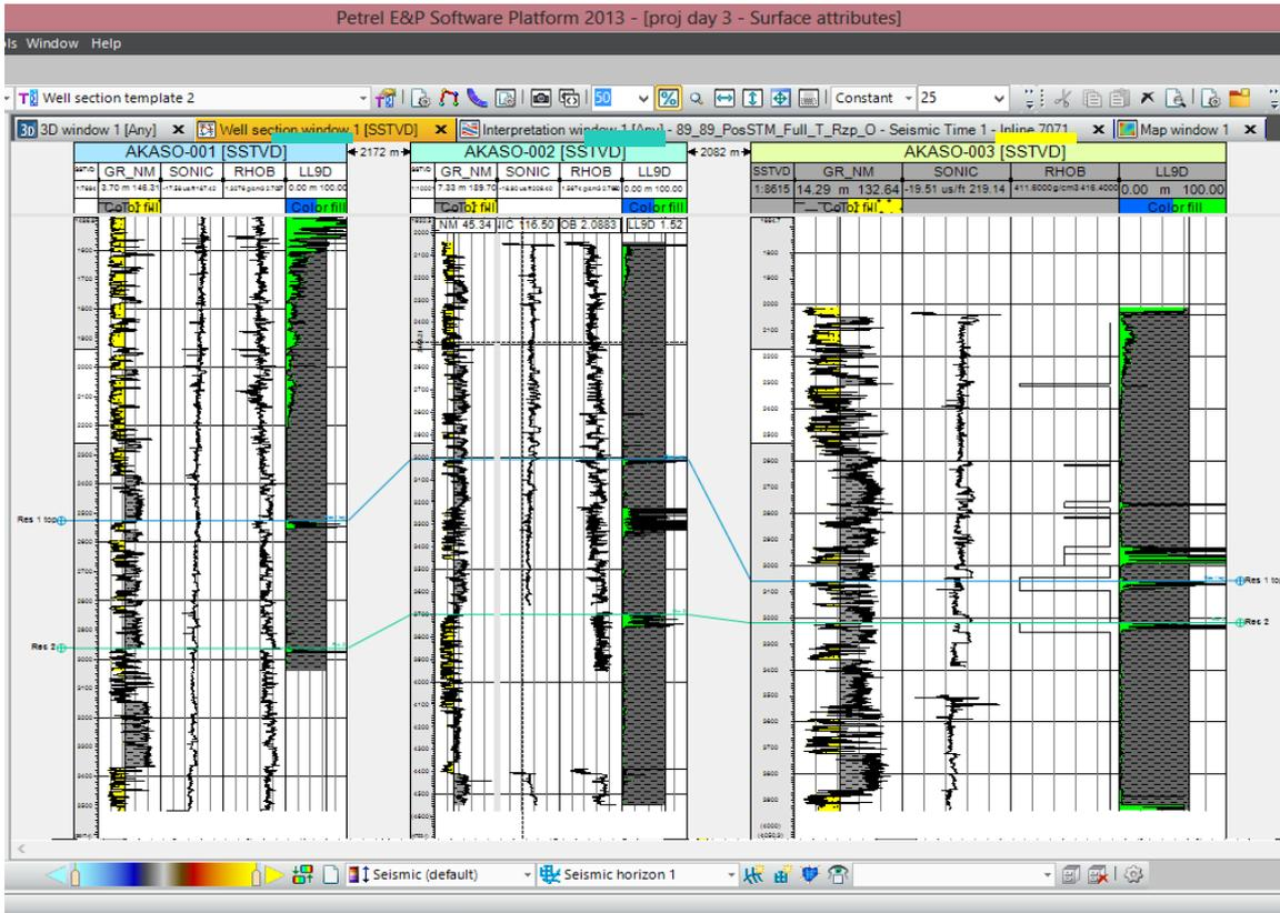
Figure 5: Wire line logs showing the stacking patterns and top-seal
