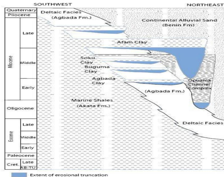
**Figure 2:** Stratigraphic column showing the three formations of the Niger Delta (Tuttle et al.1999, Modified from Doust and Omatsola, 1990).
