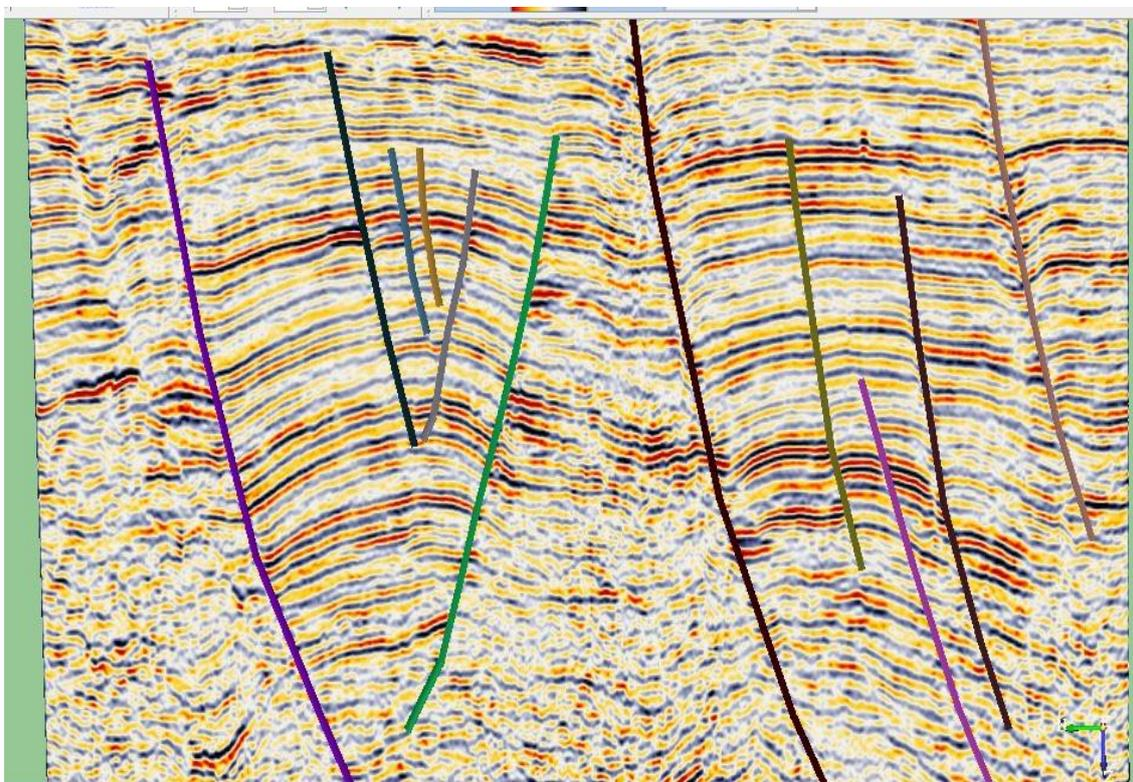
**Figure 4:** 3-D Seismic inline section showing the major synthetic growth faults. Eleven (11) faults were delineated across the field with nine (9) faults trending NW-SE while two (2) faults trend NE-SW.
